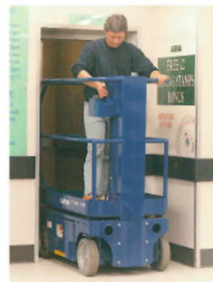
Low stowed height allows TM12 to drive through doorways with operator in platform.
